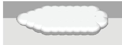
图5 船体模型的离散元构建 Fig.5 The ship hull constructed with overlapped 3D disks
